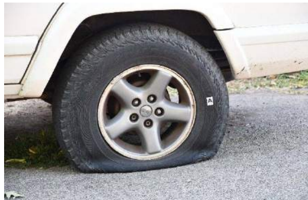
DSC_2826- Flat tire on the Jeep, rear passenger tire. Defect possibly on the interior of the tire.
