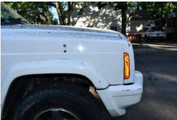
DSC_2834- Defects B and C located on the front passenger side panel.
