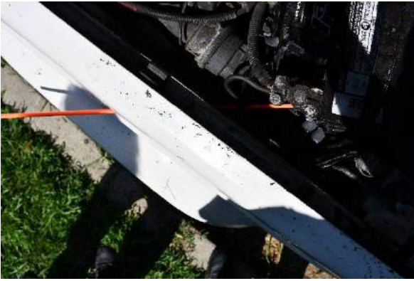
DSC_3004- Bird's eye view of defect B with trajectory rod placed in defect B and exits towards defect in the battery.
