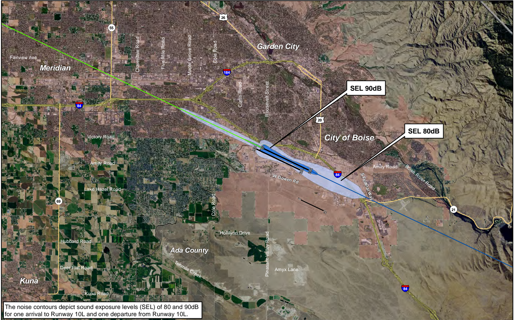
Figure B-10 Bombardier CRJ-200 Sound Exposure Level (80dB/90dB) Noise Contour
