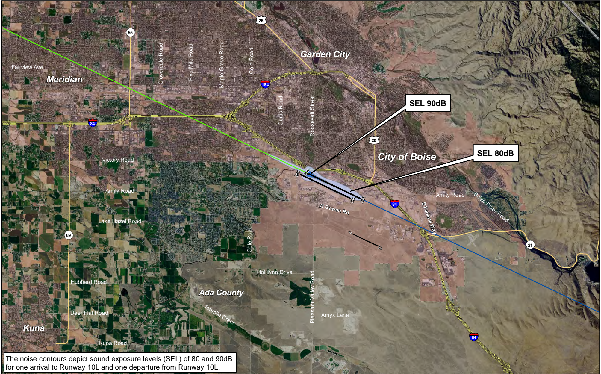
Figure B-14 Bombardier Q-400 Sound Exposure Level (80dB/90dB) Noise Contour
