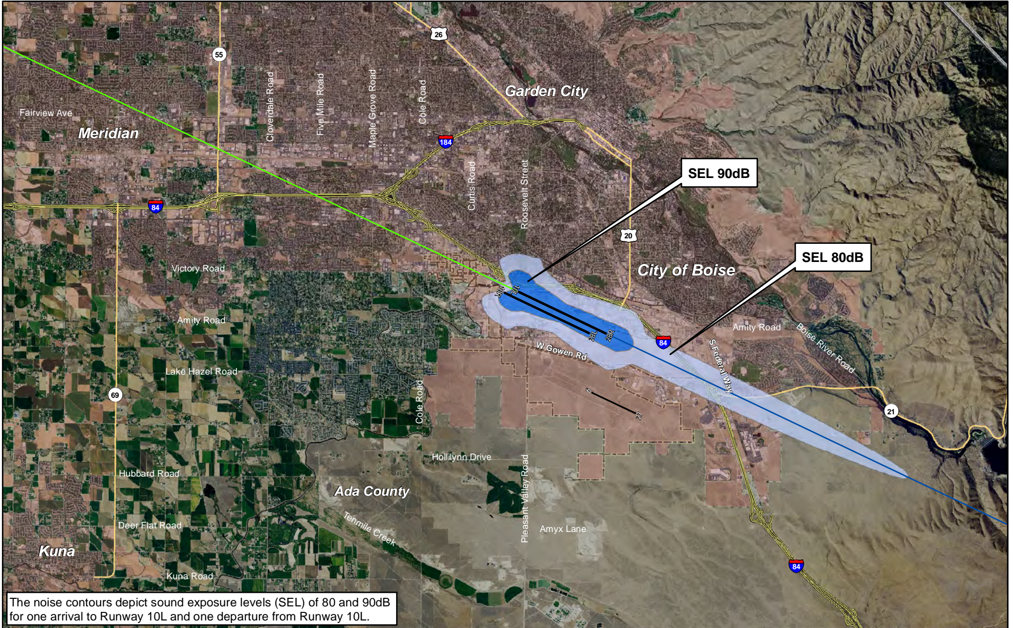
Figure B-15 Cessna 182 Sound Exposure Level (80dB/90dB) Noise Contour
