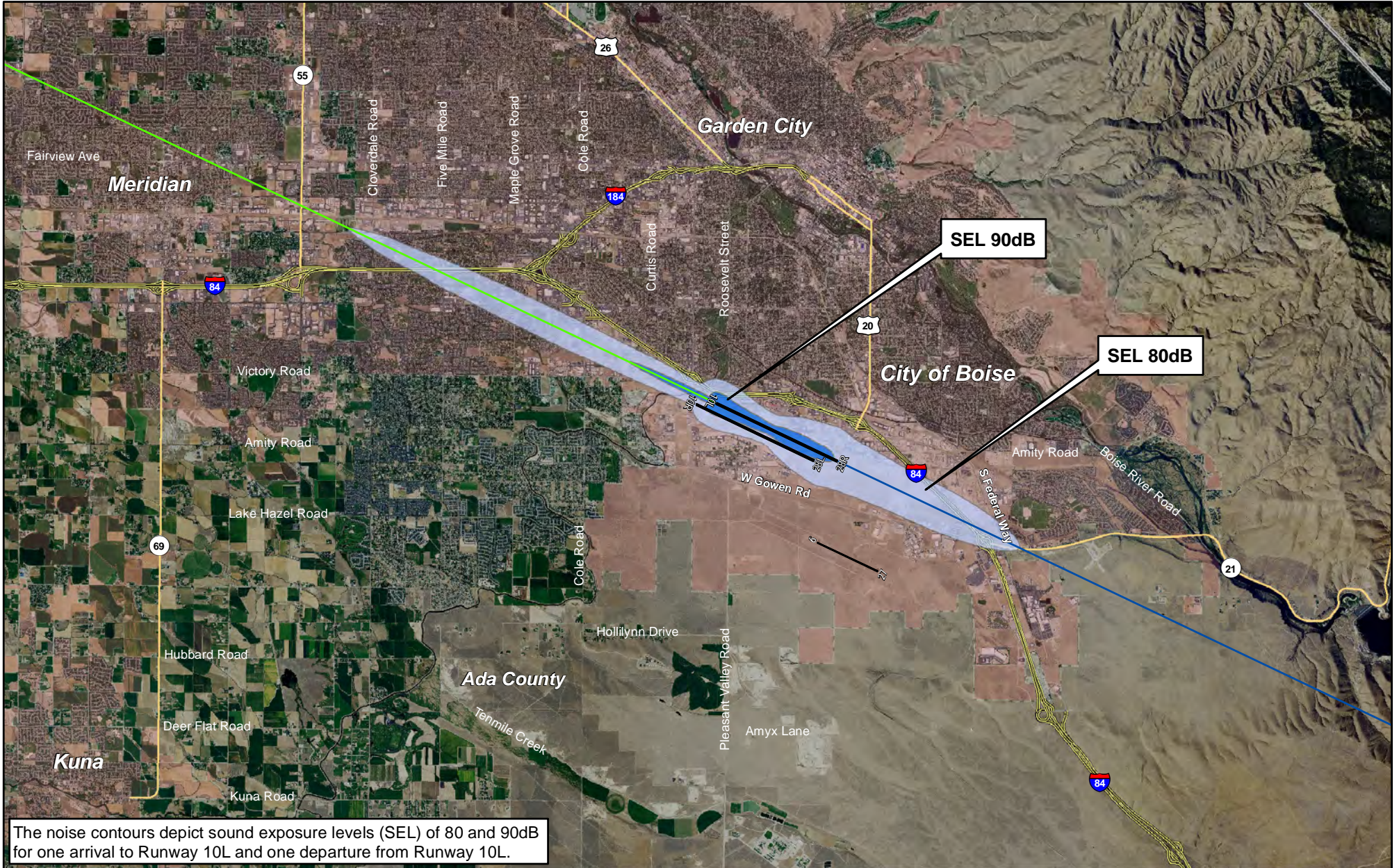
Figure B-11 Bombardier CRJ-700 Sound Exposure Level (80dB/90dB) Noise Contour
