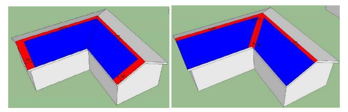
Panels/module arrays shall not be placed on the portion of a roof that is below an emergency escape and rescue opening. A pathway not less than 36 inches (914 mm) wide shall still be provided to the emergency escape and rescue opening as specified in prescriptive code.
