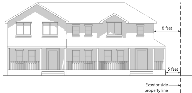
Figure 4.3. Two-Story Attached Units on Contiguous Lots - Setbacks
