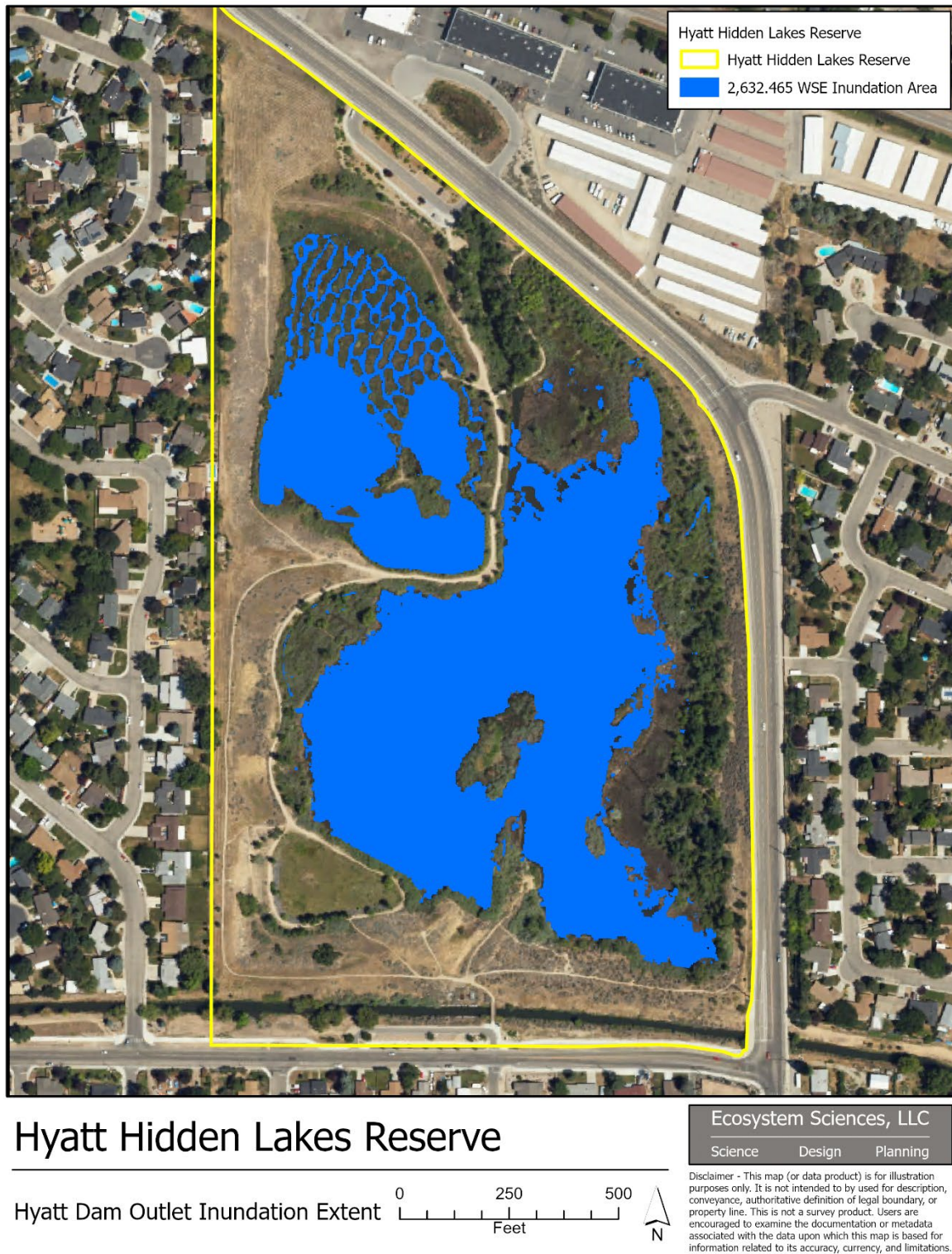
Figure 11. Inundation Extent at WSE 2,632.465 ft (Hyatt Dam).
