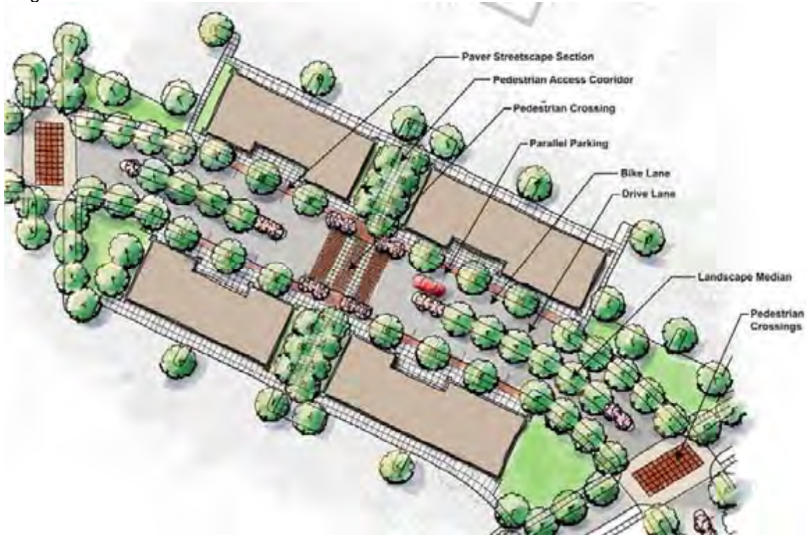
Urban core of Barber Station showing conceptual tree planting, paving design and walkway connections from adjacent parcels.
