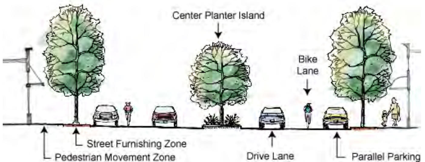
Conceptual section through Barber Station Drive showing street trees
