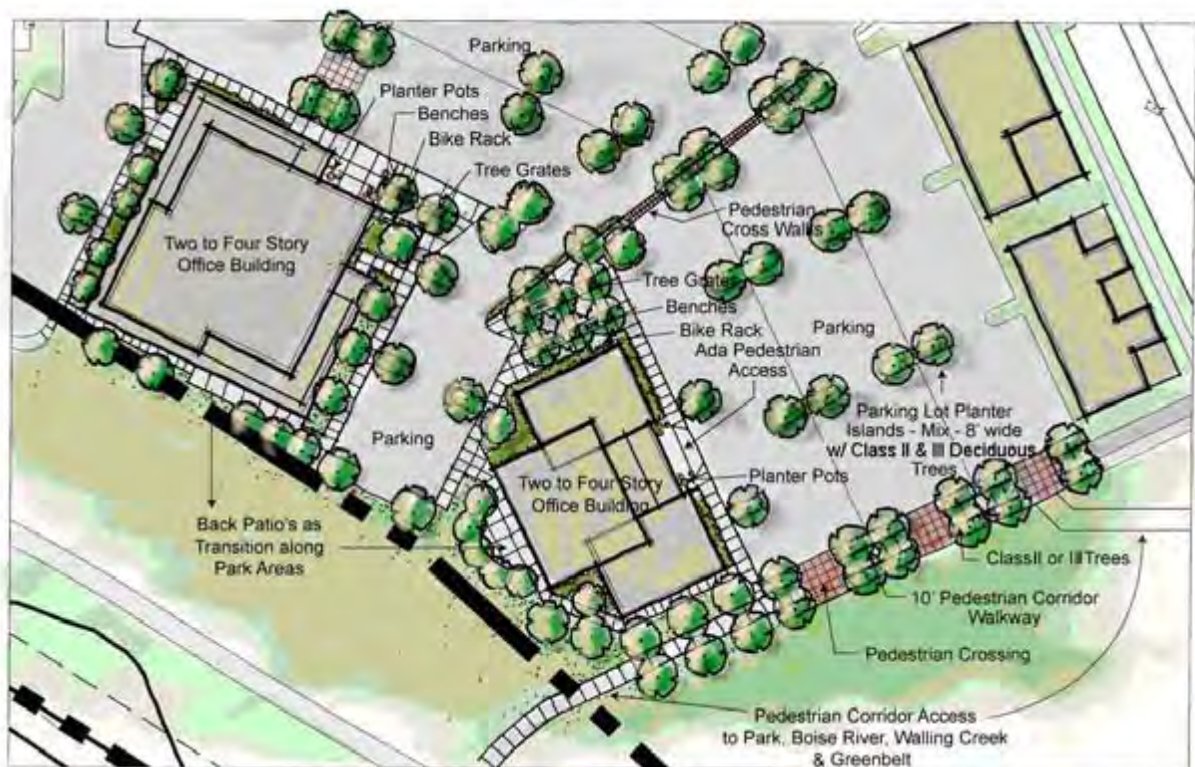
Conceptual example of design and layout of street furniture, walkways and paving.
