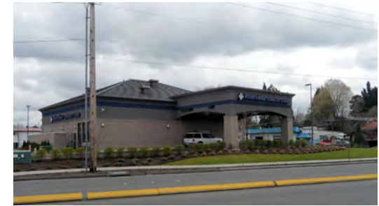
Fig. 3-10. While drive-through lanes between the street and building aren't prohibited, they count as a parking lot for the purpose of building/parking lot location standards in Chapter 2 frontage provisions. Also, the facade would need more windows to meet transparency provisions of Chapter 2 and clear pedestrian access is needed between the sidewalk and the main building entry.
