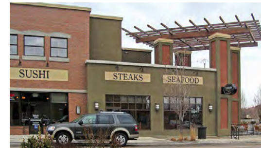
Fig. 4-26. Example of vertical building modulation combined with a change in materials.
