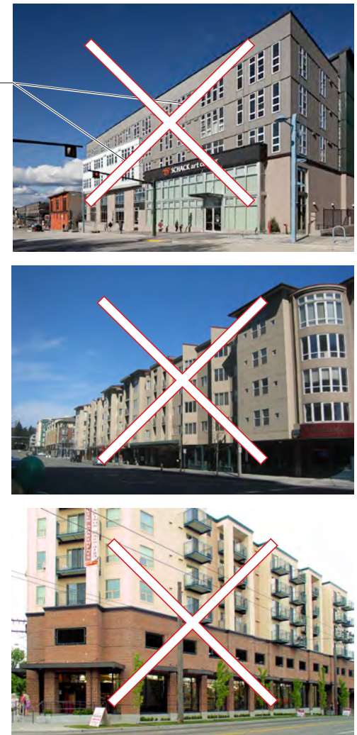
Fig. 4-22. Examples where facade widths are greater than 130 feet and do not include acceptable techniques to break up the facade's mass.
