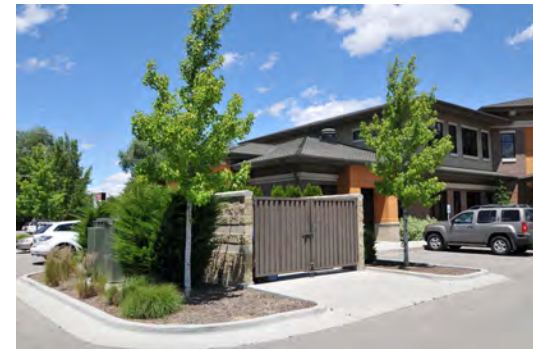
Fig. 3-17. Service enclosure examples. In the top image, service elements are hidden behind the gates and wheeled out on trash days.
