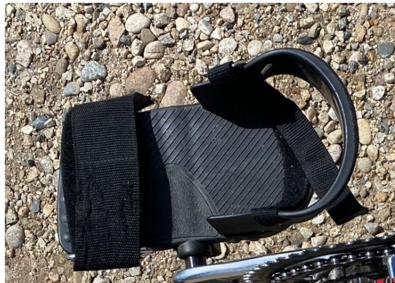
Adaptive foot pedals with ankle and toe straps, found on our recumbent trikes
