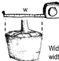
Width of hole should be 2-3 times the width of the root ball
