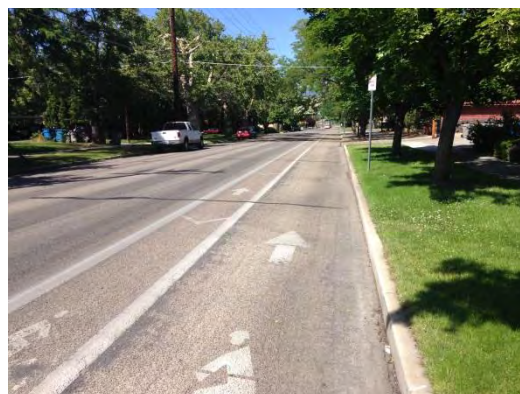
Adding a Buffer to a Bike Lane Can Help Create a Low-Stress Bike Route
