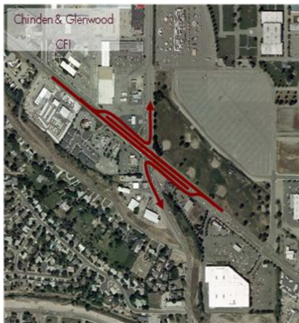
Figure 2-10: Continuous Flow Intersection
